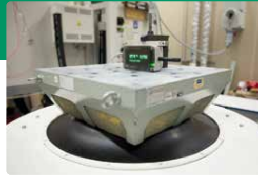
The Shaker System is one of the types of test equipment we use for environmental testing
