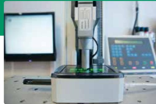
One example of materials testing is steady force, which is part of our safety analysis of electronic devices
