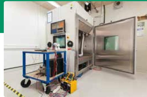
HALT is a progressive method for improving product quality and for reducing failure rates and warranty costs
