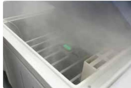
Salt mist testing is a proven method to verify if your product is corrosion resistant
