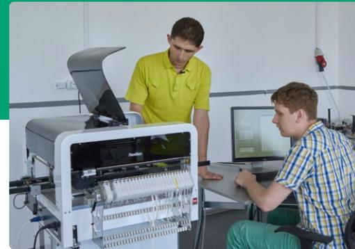
Flexible prototype pick and place machine.
